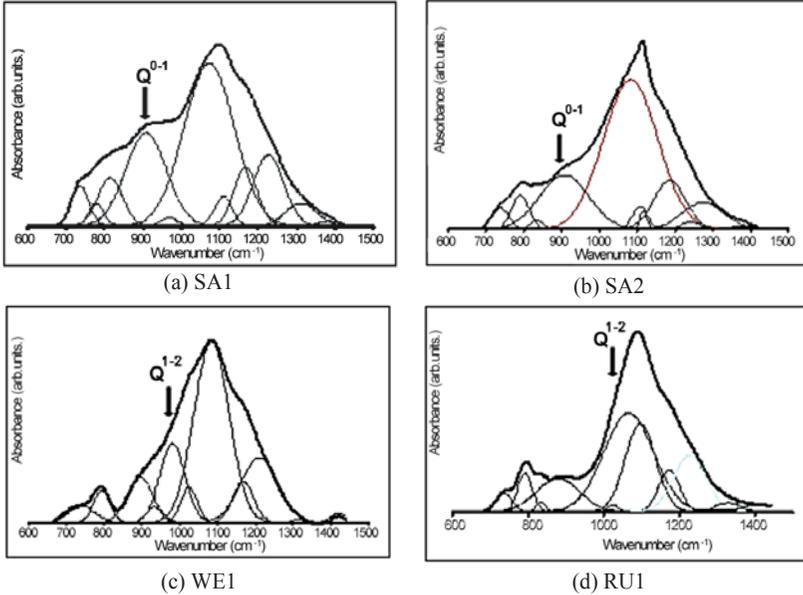
**Figure 2:** The deconvolution profile of IR-spectra for investigated fly ash (the range of wave numbers 650-1350  $\text{cm}^{-1}$ ):  $Q^{0-1}$  – Si-O-Si bonds associated with silicate of ortho- and diortho- groups;  $Q^{1-2}$  – Si-O-Si bonds associated with diortho-chain silicates
