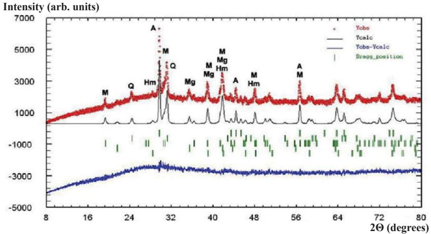
**Figure 1:** Calculated X-ray spectrum for fly ash WE1A – anatase (standard), M – mullite, Q – quartz, Mg – magnetite, Hm – hematite.
