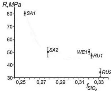
**Figure 3:** The compressive strength (R) of fly ash based geopolymer binder vs. polymerization degree of vitreous phase
