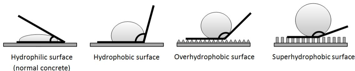
**Figure 1.** The hydrophilic ( $0^\circ \leq \theta \leq 90^\circ$ ), hydrophobic ( $90^\circ \leq \theta$ ), “over-hydrophobic” ( $120^\circ \leq \theta < 150^\circ$ ) and superhydrophobic ( $150^\circ \leq \theta \leq 180^\circ$ ) surfaces, where  $\theta$  is the CA.
