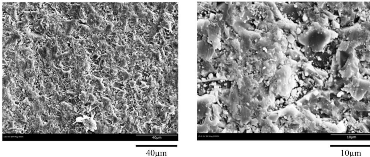
26 **Figure 10.** The surface of mortar tiles observed by SEM at 500x (left) and 2000x (right)
