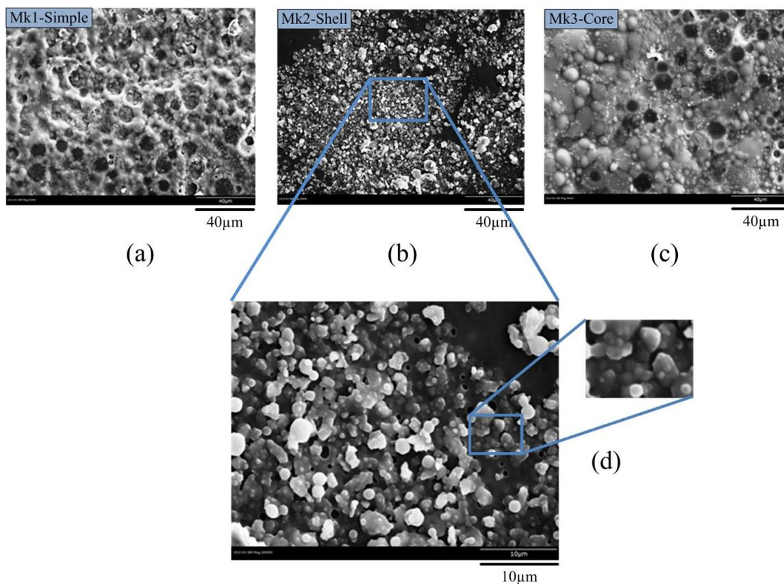
**Figure 12.** SEM images of superhydrophobic coatings at 500x magnification for: a) Mk1; b) Mk2; c) Mk3; and d) Mk2 at 2000x magnification.
