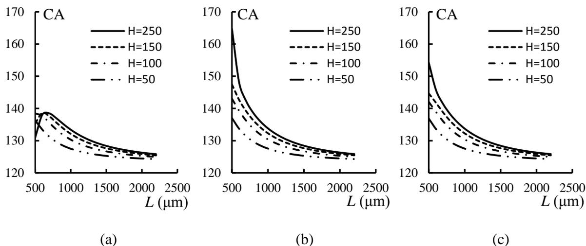
**Figure 17.** CA versus distance of the aggregates,  $L$ , for  $D=500 \mu\text{m}$ ,  $R_{fc}=1$  and  $\theta_a = \theta_c \approx 95^\circ$  (a)  $n=30$  and  $d=2 \mu\text{m}$  (Mk1) (b)  $n=100$  and  $d=5 \mu\text{m}$  (Mk2) (c)  $n=20$  and  $d=10 \mu\text{m}$  (Mk3)
