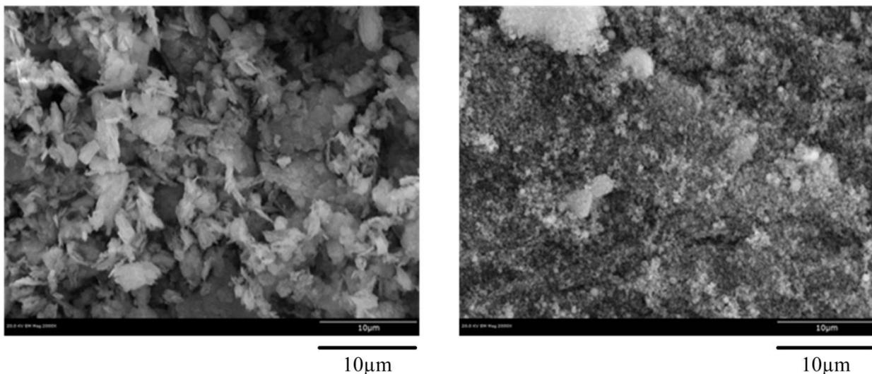
**Figure 6.** SEM images of metakaolin (left) and portland cement (right), (2000x magnification)
