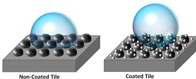
**Video of water droplet on superhydrophobic concrete**
