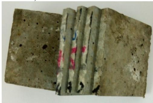
**Figure 1.** Cut plates of exposed cement sample
