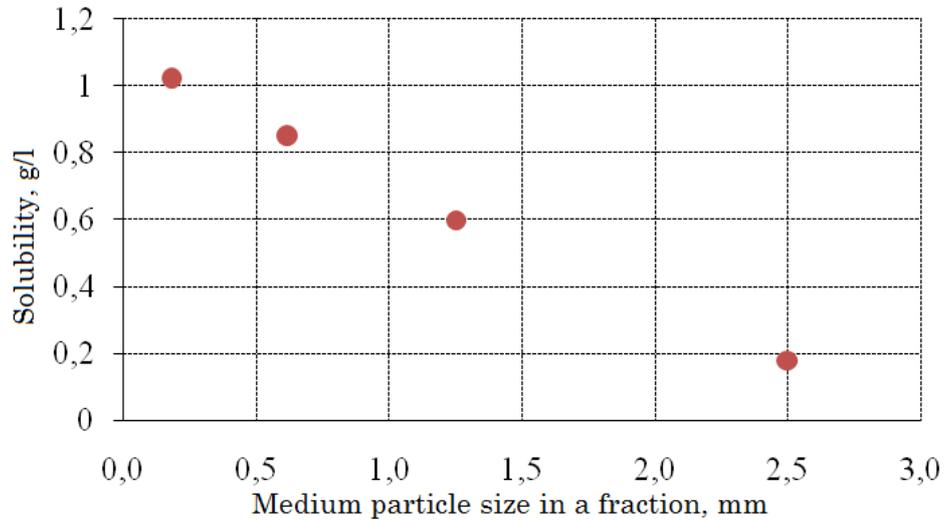
**Figure 1.** The dependence of the solubility of gypsum on particle size (Bazhenov et al., 2012; Lesovik, Ginzburg & Volodchenko, 2014)
