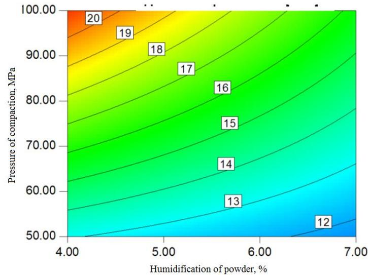
**Figure 4.** The strength at compaction of the samples from the pressed gypsum particles depending on the moisture content of the material and pressure of compaction (test conditions: storage temperature of samples: 20 °C, storage time: 7 days, without the use of a plasticizer)
