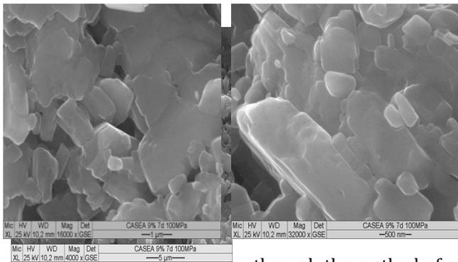
**Figure 5.** Merging of gypsum particles of the pressed samples (conditions: ground natural gypsum, pressure of compaction 100 MPa, water-gypsum ratio - 0,09, storage in closed containers - 7 days)
