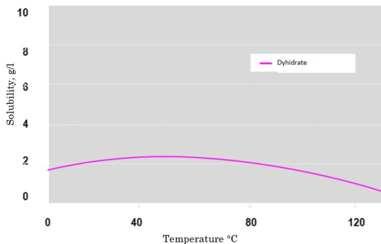
**Figure 2.** The dependence of the solubility of calcium sulphate dihydrate (gypsum) on temperature
