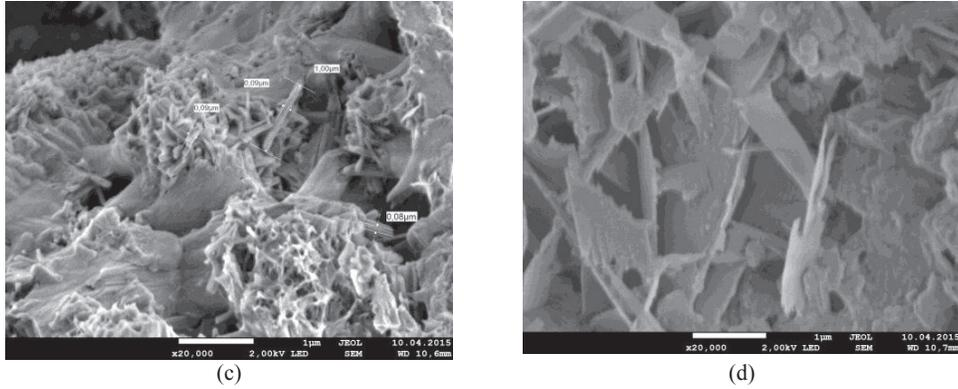
**FIGURE 3.** The microstructure of inter-pore partitions of autoclaved foam concrete
