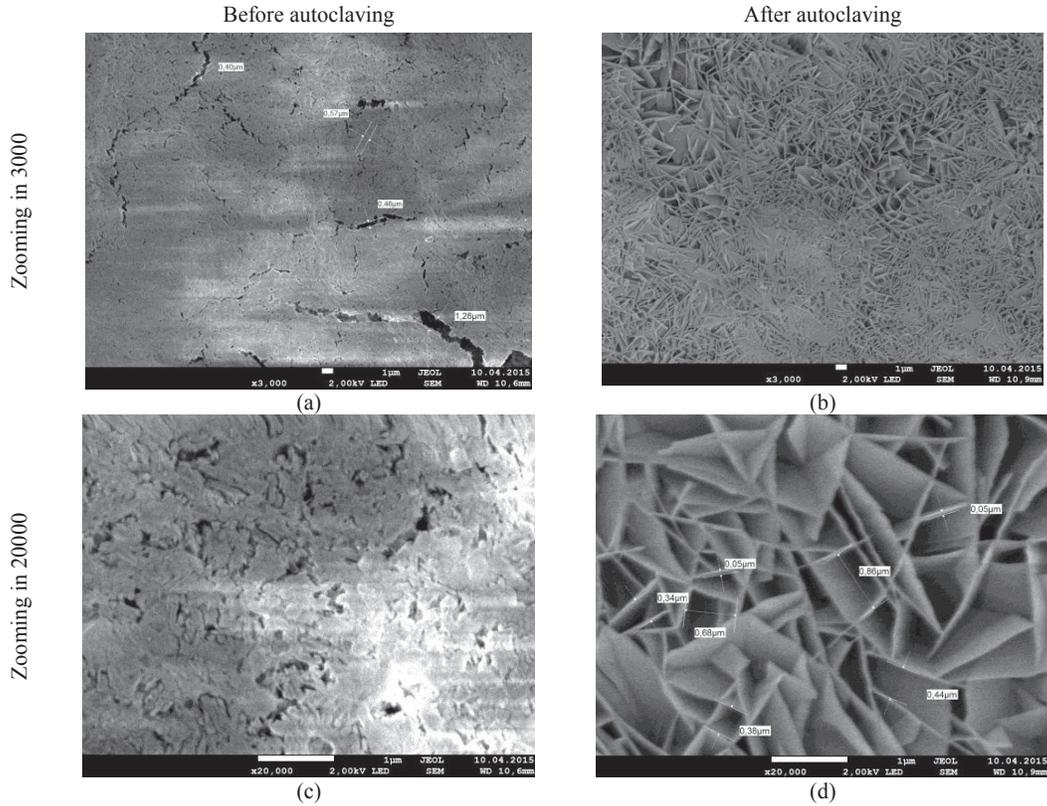
FIGURE 2. The microstructure of the interpore surface in foam concrete
