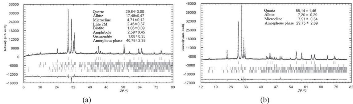
FIGURE 1. Data of quantitative full-profile XRD-analysis of sands, wt. %:
