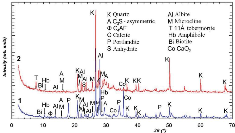
**FIGURE 4.** Diffraction pattern of foam concrete: 1 – cured in ambient conditions, 2 – cured under autoclaving
