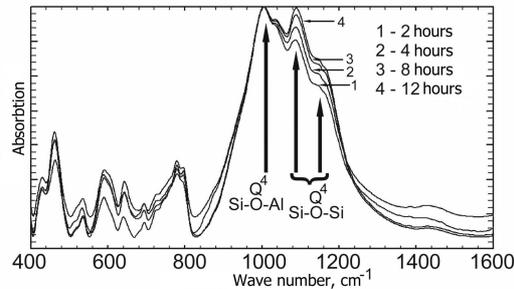
**Fig. 3. Superposition of normalized infrared absorption profiles for the binder with a various mechanical activation time**
