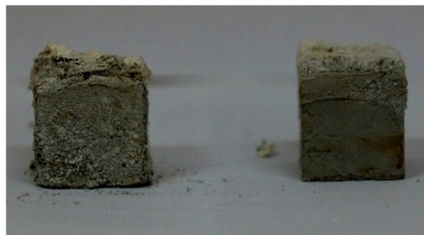
Figure-5. Blooms at surface of perlite geopolymer samples based on Na 2 SiO 3 .
