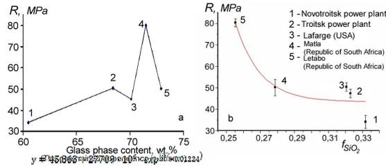
**Fig. 5. GPB compression strength for various fly ashes as a function of phase (a) and phase -dimensional heterogeneity (b).**
