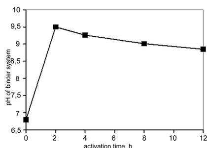
**Fig. 1. Dependence of pH of the synthesized binder system on a mechanical activation time**
