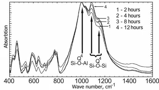
**Fig. 3. Superposition of normalized infrared absorption profiles for the binder with a various mechanical activation time**
