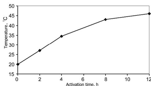
**Fig. 2. Dependence of the synthesized binder system temperature on a mechanical activation time**
