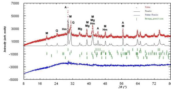
**Fig. 4. Result of the USA fly ash roentgenogram calculation.**
